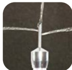
Tri-Port Discharge (end & side ports injection)
